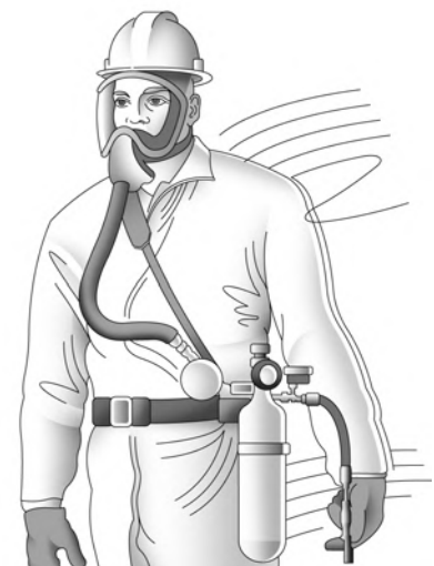
Tight-fitting Atmosphere-Supplying Respirator with an auxiliary escape bottle APF=10,000 in escape mode only; otherwise APF=1,000 Full facepiece Needs to be fit tested
