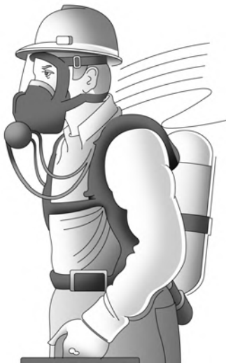
Tight-fitting Self-Contained Breathing Apparatus (SCBA) pressure-demand mode APF=10,000 Demand mode APF=50 Needs to be fit tested
