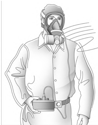
Tight-Fitting Full Facepiece Powered Air-Purifying Respirator (PAPR) APF=1,000 Needs to be fit tested
