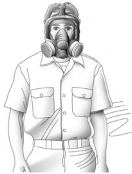
Full Facepiece Elastomeric Respirator APF=50 Needs to be fit tested
